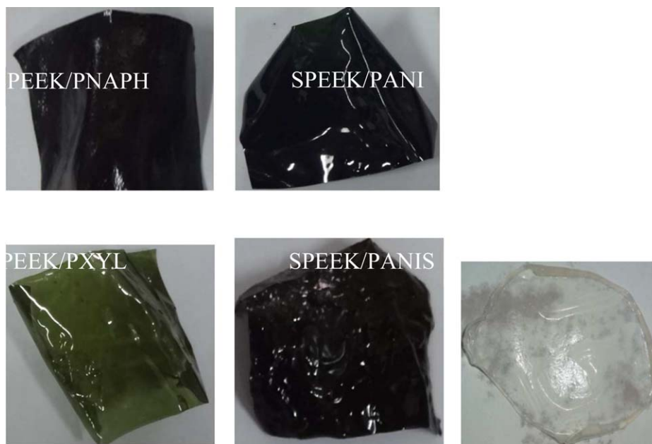
Figure 12. Hydrolytic stability of the membranes at elevated temperature. [Color figure can be viewed in the online issue, which is available at wileyonlinelibrary.com.]
